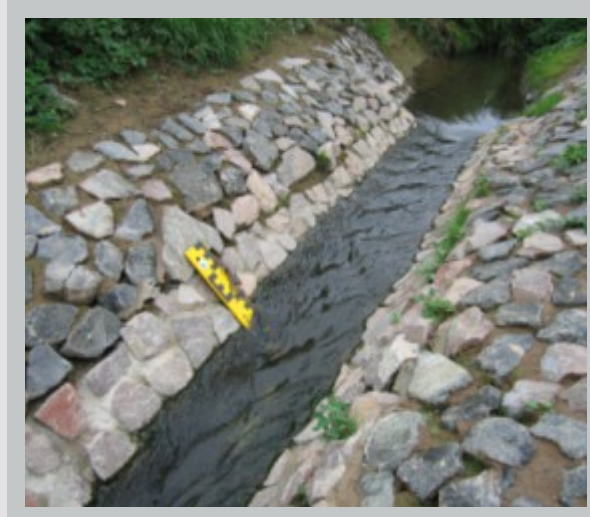
Measurement point with gauge staff
