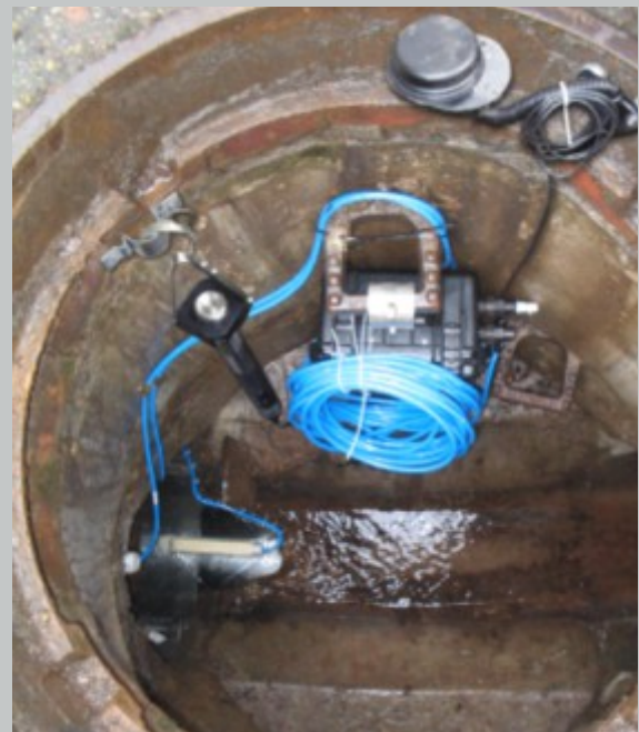
Measuring instrument with data transmission via GPRS
