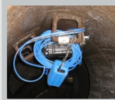
Measurement place in channel Transmitter with data logger in manhole
