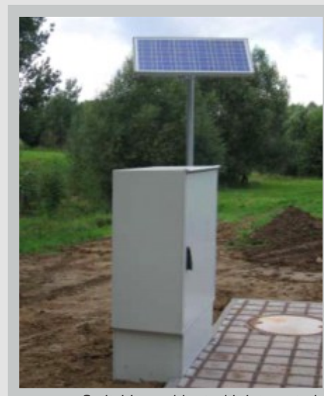
Switching cabinet with integrated data logger and solar panel
