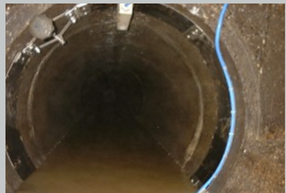
Flow measurement point
