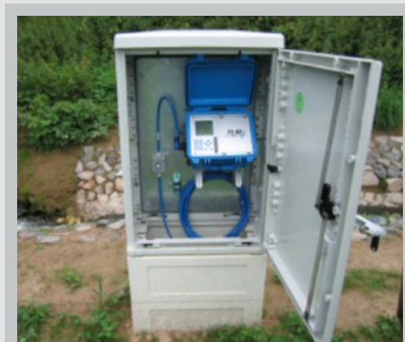
Open switching cabinet with transmitter
