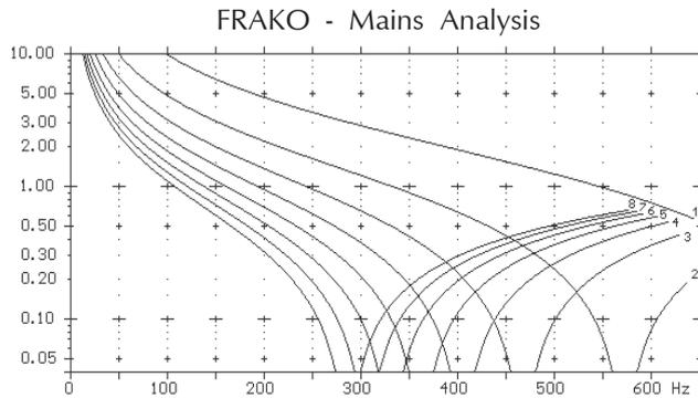
When the power correction system is fully switched in, an impedance factor of  $\alpha^* \geq 0.5$  will only suffice for a remote control frequency of 166 Hz.
