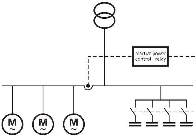
**Fig. 28: Incorrect!** The current transformer only registers the load current: the capacitor bank is switched in but not out again. Automatic calibration of the reactive power control relay is not possible!
