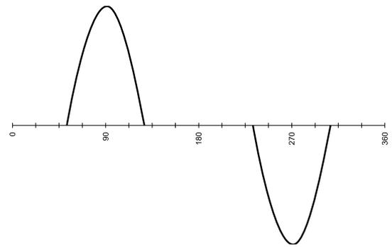
**Fig. 32:** Current of a power rectifier
