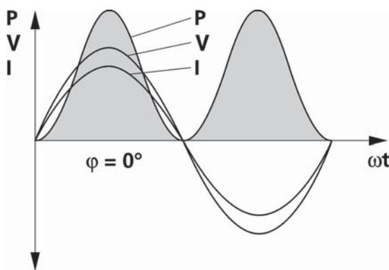
Active or real power is that component of the power that is converted into another form (e.g. heat, light, mechanical power) and is registered by the meter.
