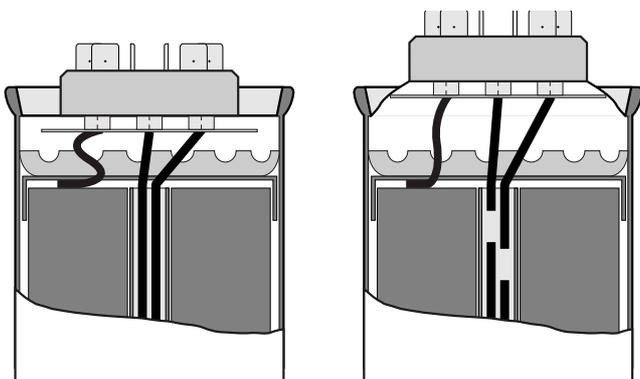
FRAKO power capacitors therefore offer a high degree of safety when overloaded and at the end of their service life.
