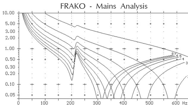
With the power factor correction system switched in, an impedance factor of  $\alpha^* \geq 0.5$  is achieved with certainty for a remote control frequency of 216.7 Hz.
