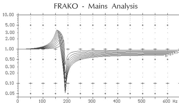
*Choking reduces the resonance frequency to a value below 250 Hz. All harmonics above the resonance frequency of the choked system are attenuated.*
