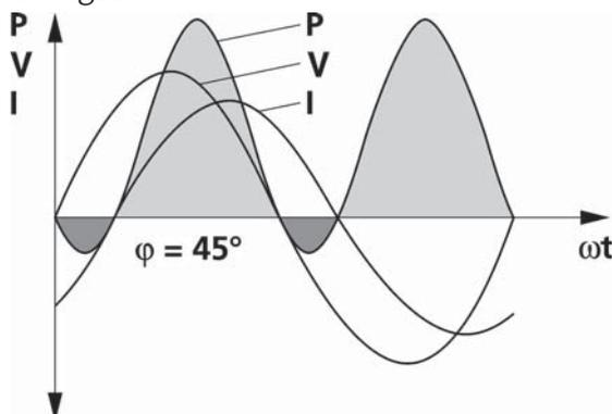
In this example phase displacement  $\varphi = 45^\circ$  has been chosen. This corresponds to an inductive  $\cos \varphi$  of 0.707. Part of the power curve can be seen to be in the negative area.
