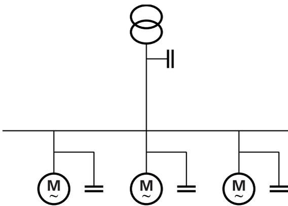
**Fig. 8:** Typical individual power correction
