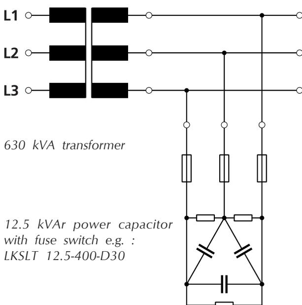
The capacitor with fuse switch can be directly connected to the terminals of the transformer. This means that the lines to the capacitor must be dimensioned for the full short-circuit power.
