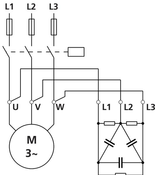
25 kW induction motor running at 1500 min<sup>-1</sup> 10 kVAr power capacitor e.g.: LKN 10-400-D32
