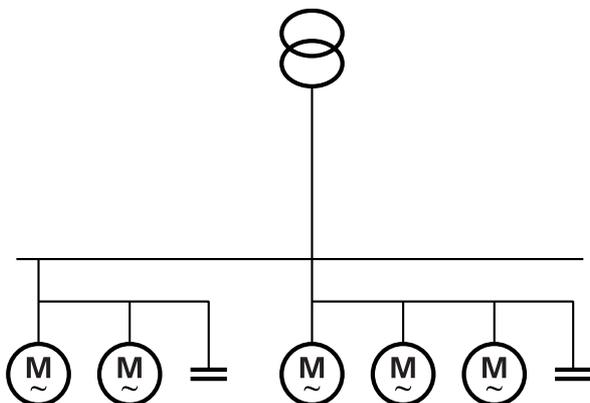
**Fig. 9:** Typical group power factor correction
