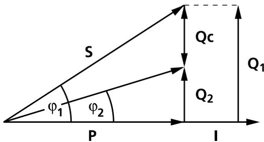
The reactive power  $Q_c$  corrected by the capacitor is given by the difference between the inductive reactive power  $Q_1$  before correction and the reactive power  $Q_2$  after correction, i.e.  $Q_c = Q_1 - Q_2$ .
