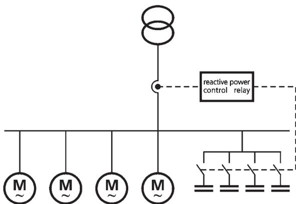
**Fig. 10:** Typical central power factor correction system
