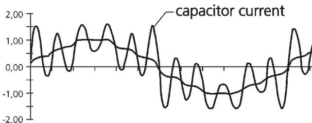
If, for example, about 7% of the 11th harmonic is present, then the voltage is 7% higher, but the effective level of the capacitor current is 1.33 times the capacitor nominal current! For this reason a high current-carrying capacity is even more important than the overvoltage capacity.
