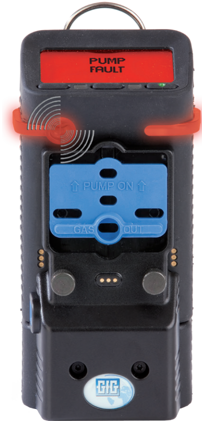
G460 with pump activated: - Sensor cover UP - Diffusion inlets covered
