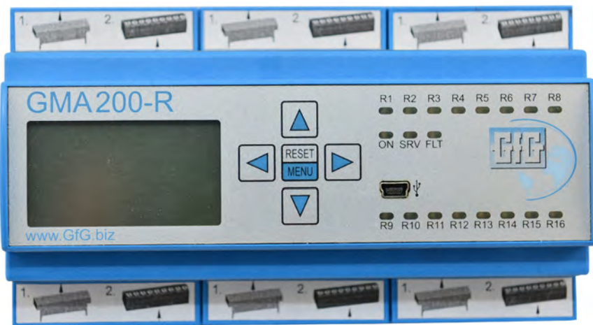
GMA200-RTD with a display for remote measured value display
