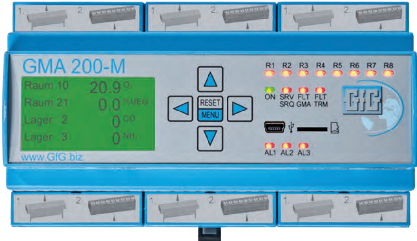
GMA200-MT 6 with a display for quick and safe evaluation
