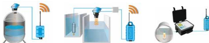
**Example:** Ultrasonic level measurement in Ex zone, Data logger and GPRS transmission
