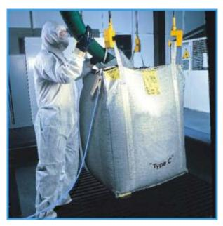
and it sets out the essential requirements of Type C bags in relation to eliminating the risk of charge accumulation on the bag. It states that the resistance through the bag should be less than 1 x 10<sup>7</sup> ohms (10 meg-ohm). This means that the resistance from a point on the bag to a grounding tab should never be higher than 10 meg-ohm. The latest edition of NFPA 77, "Recommended Practice on Static Electricity", recommends this value of resistance.
