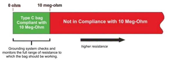
Likewise, if a company is committed to using IEC / NFPA 77 compliant 10 meg-ohm bags the permissive range of resistance to which the grounding system should be monitoring should be 0 ohms up to 10 meg-ohms.
