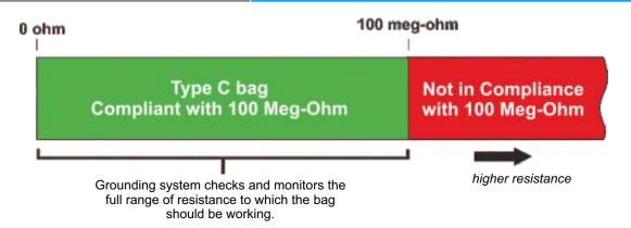
This ensures that bags of different static dissipative consistency can be checked and monitored for the full permissive range of resistance. Any bags operating outside of this range should be rejected.
