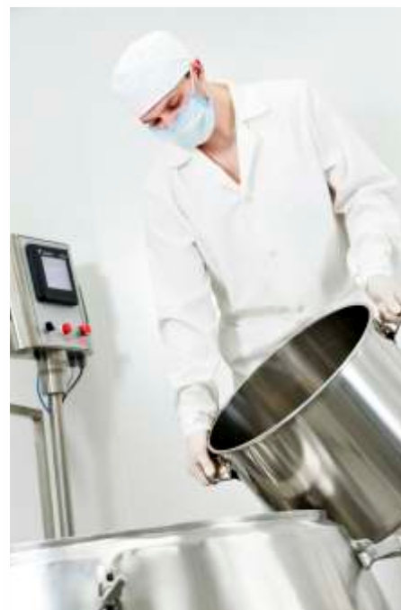
Fig. 1. A blender getting charged with a powder. Note that the bucket discharging the powder should be bonded to the receiving vessel or grounded independently.
