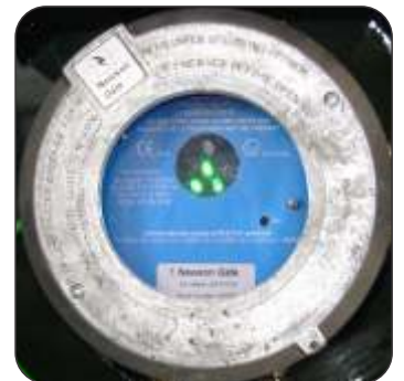
Fig. 3 Earth-Rite® PLUS ground status indicators pulse continuously when grounding is in place.
