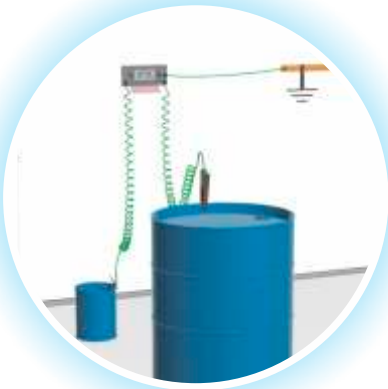
Grounding of drums with clamps and Hytrel anti-static retractable spiral cable (more detail overleaf)
