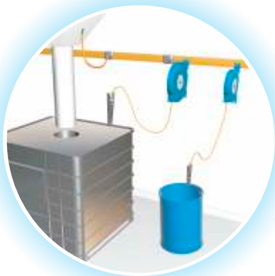
Grounding of metal IBCs and drums with clamps and retractable reels (more detail overleaf)
