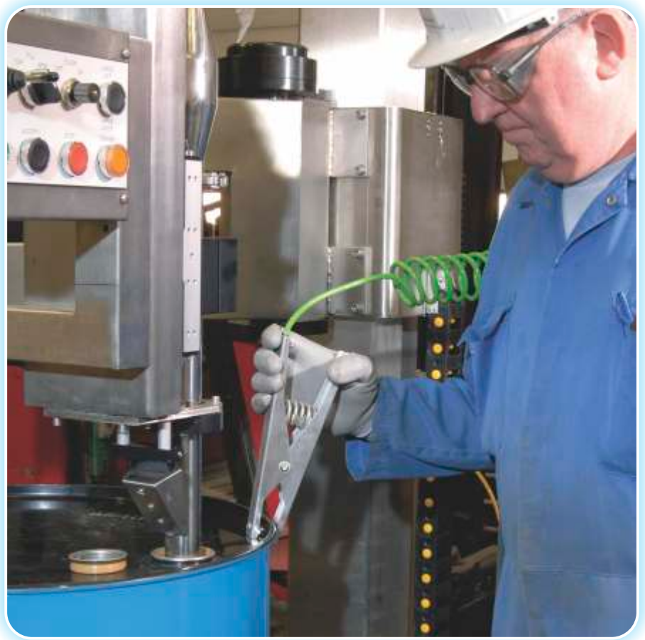
Cen-Stat clamps are designed to penetrate through coatings, hardened product deposits, rust and dirt to enable low resistance electrical connections to safely dissipate static electricity
