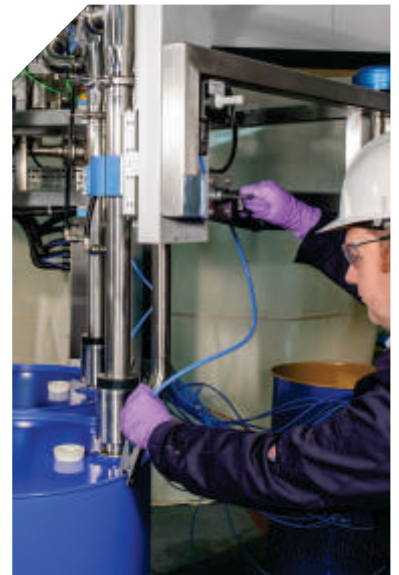
Fig. 2: Pulsing green ground status indicators provide operators with a visual reference point to ensure the equipment they are operating is grounded prior to, and during, the operation.
